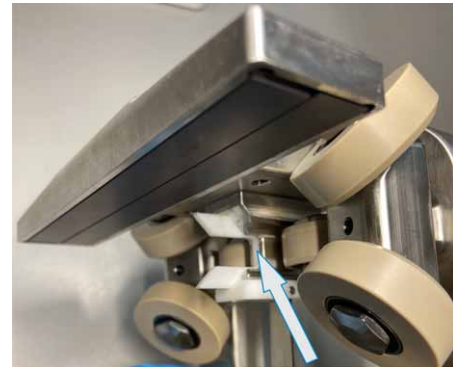
Lubrication block mounted on lubrication shuttle
