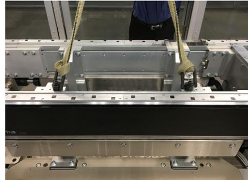
3. Use an appropriate lifting device, such as a forklift, to lift the straight section by the middle of the lifting strap.
