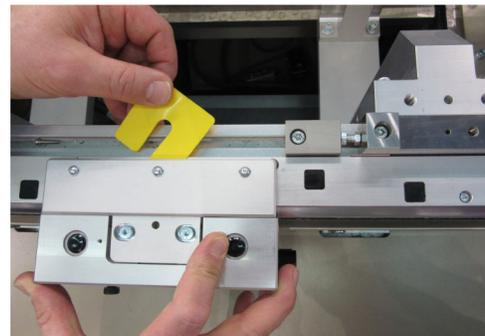
2. If the gap is greater than 0.5 mm (0.02 in.) +/- 0.3 mm (0.01 in.), verify that the shuttle shim is the problem (not the v-wheels or shuttle encoder strip assembly):
