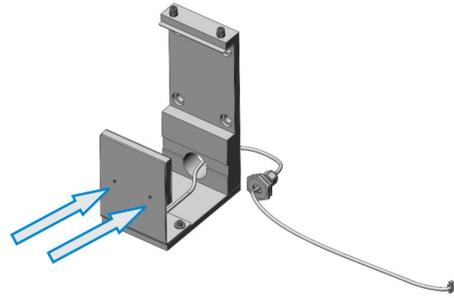
2. Route the IR reader cable through the IR reader mount assembly cable opening.
