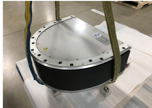
3. When the 180 deg. section is in the required position, remove the lifting straps.
