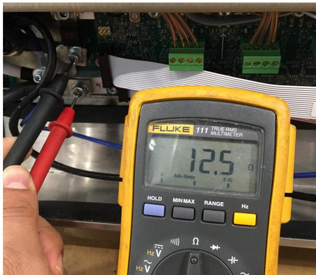
2. Look at the value displayed on the multimeter screen and determine if the resistance is acceptable:
