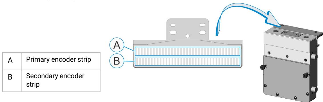
Align a shuttle encoder strip assembly if the encoder strip is removed during maintenance, or if the shuttle position faults regularly occur on the curved section.
