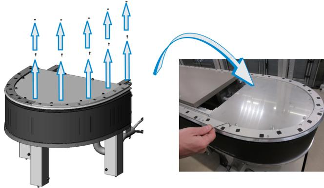
4. Remove the five (5) encoder assembly screws.
