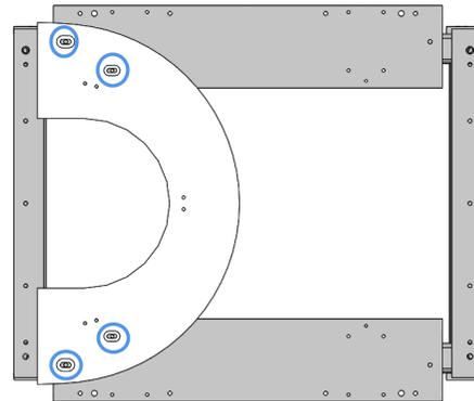
2. Lift and position a 180 deg. section on the 180 deg. plate.
