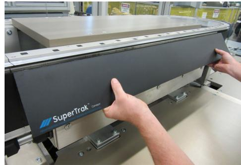
3. Slowly tilt the motor cover label toward the motor until it is adhered to the motor.
