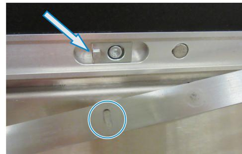
5. Release the flat wear strip. The channel magnets pull the flat wear strip into the channel.
