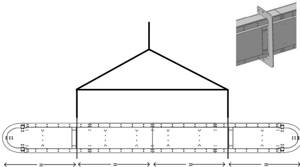
1. Remove from shipping box using the upper two holes on each lifting bracket. Use of a spreader bar is required.
