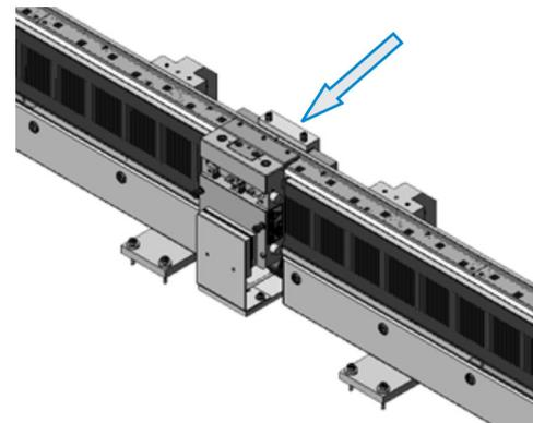
4. Tighten the two (2) clamp screws, to hold the IR reader mount in position.
