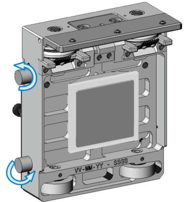
3. Align the replacement bumper threads with the bumper spacer (if used) or with the bumper hole on the shuttle.
