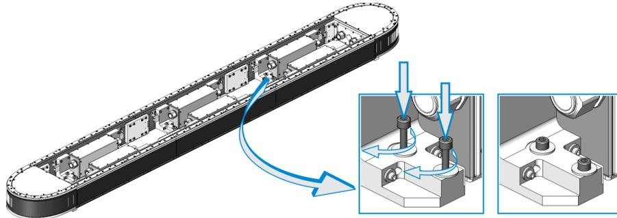
16. Add wear strip locators to straight sections with the tabs directed towards the center of the each section.
