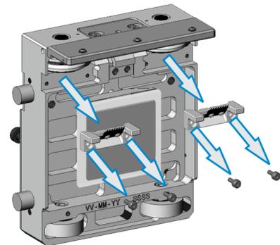
5. Remove the two (2) plastic caps on the top of the shuttle.
