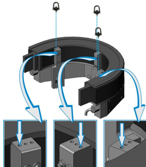
2. Attach one (1) strap to each of the three (3) M8 rotating eye bolts.
