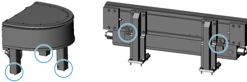
4. Install two (2) dowels through the outer holes of top connection plate, to position the top connection plate on the frame.
