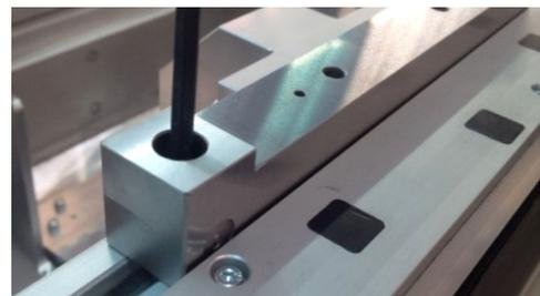
5. Position an adjust block at the end of the stationary mount, and secure it in position with one (1) screw.
