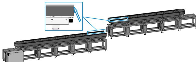
In this procedure, “section A” references an installed straight section, 180 deg. section, or group of sections. “Section B” is the straight section, 180 deg. section, or group of sections being installed next to section A.
