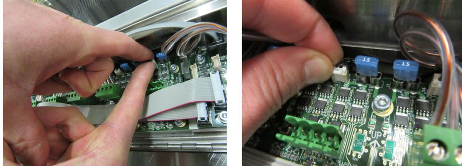
6. Pull the old thermistor wire straight out from the thermistor hole.
