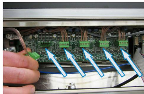
6. Remove the fourteen (14) screws that secure the coil driver board to the bus bar.
