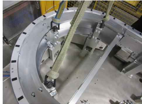
3. Use an appropriate lifting device, such as a forklift, to lift the 180 deg. section up by the ends of the lifting straps.
