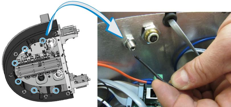
6. Slide the end of the new thermistor wire into the thermistor hole until you feel resistance.
