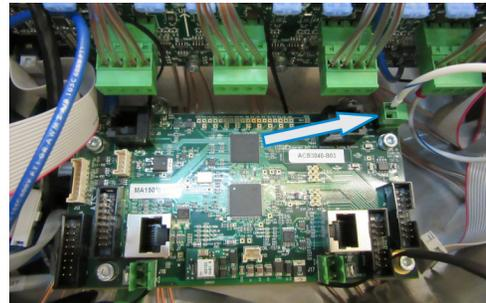
9. Remove the four (4) connection screws.
