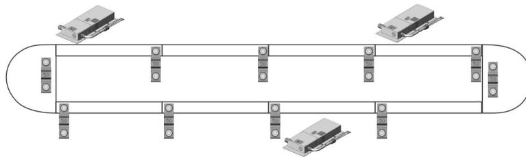
If possible, install the power supplies on the sections with the highest performance demands.
