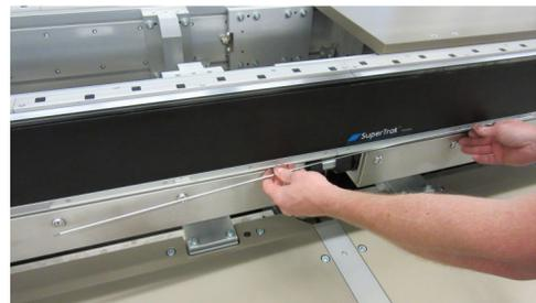
4. Remove any dirt or debris from the flat wear strip channel.
