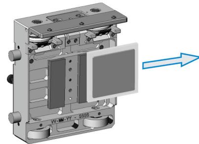
3. Install the shuttle removal tool on the shuttle:
