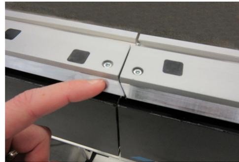
5. **If you feel a ridge, or if the shuttle makes any knocking sounds as it rolls over the upper v-rail joint**, continue with the steps in the *Adjust the Upper V-Rail  $\pm 0.05$  mm ( $\pm 0.002$  in.) Straight to Straight* or *Straight to Curved* instructions that follow immediately below.
