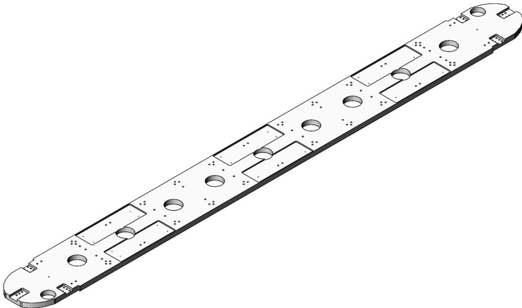
2. Position the base plate across two (2) or more metal saw horses, with the slotted cut-outs facing up.
