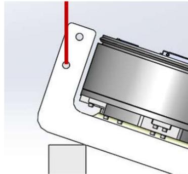
5. Lift into vertical position. As mentioned previously, use of a spreader bar is required.
