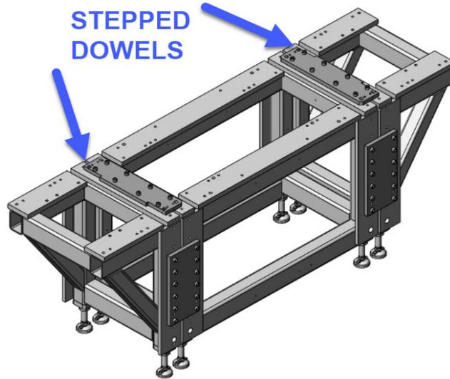
5. Install four (4) screws in the top connection plate to secure it in position.
