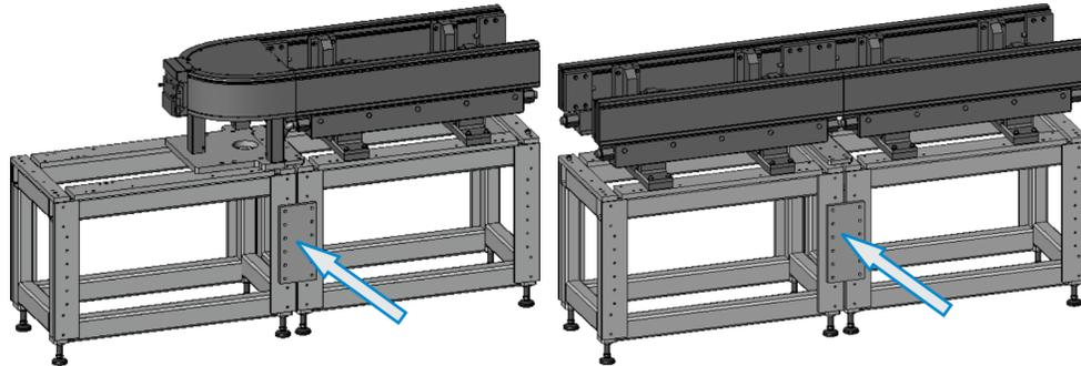
7. Use a 0.5 mm (0.02 in.) shim to verify that a 0.5 mm (0.02 in.) space exists between the aluminum surfaces of section A and section B.
