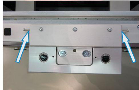
5. Install the shuttle below the removable locate.
