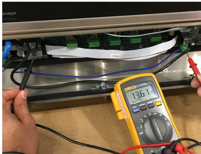
2. Look at the value displayed on the multimeter screen and determine if the resistance is acceptable:
