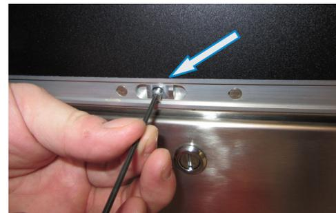
4. Align the flat wear strip slot with the locator tab.
