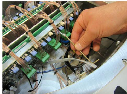
7. Disconnect the three (3) thermistor connections.
