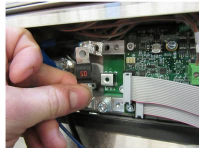
7. Install a screw through each of the two (2) 28VDC motor power connections and into the 50A fuse.
