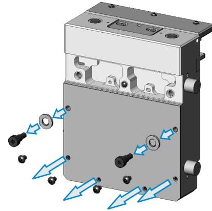
3. Remove the front cover plate from the shuttle.
