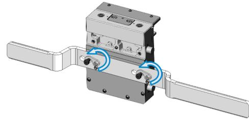
3. Pry or tilt the shuttle away from the motor: firmly hold both shuttle removal tool handles, and then pull the right handle while resisting with the left handle
