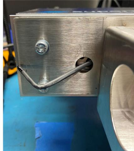
5. Replace the thermistor at the end of the wire.
