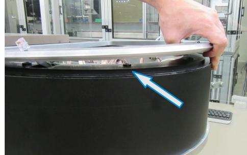
3. Install eleven (11) screws to secure the top plate in position.
