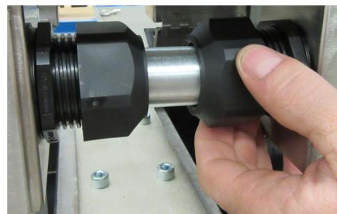
4. Feed the required wiring through the metal conduit and connect as required, then close the sections' electrical doors.
