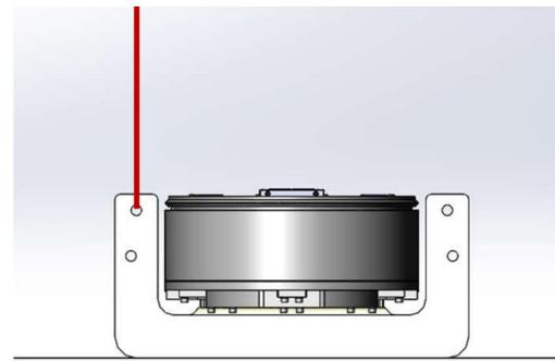
3. Lift so that the lower lifting hole is accessible.
