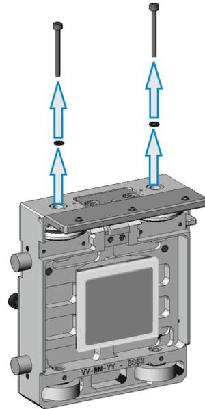
8. Attempt to manually pull the v-wheel shaft out. If snug, thread a dowel puller into the shaft and pull the shaft out.
