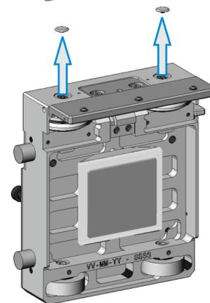
6. Remove the screw and washer that secures the v-wheel in position.
