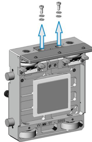
6. Lift and remove the shuttle encoder strip assembly.
