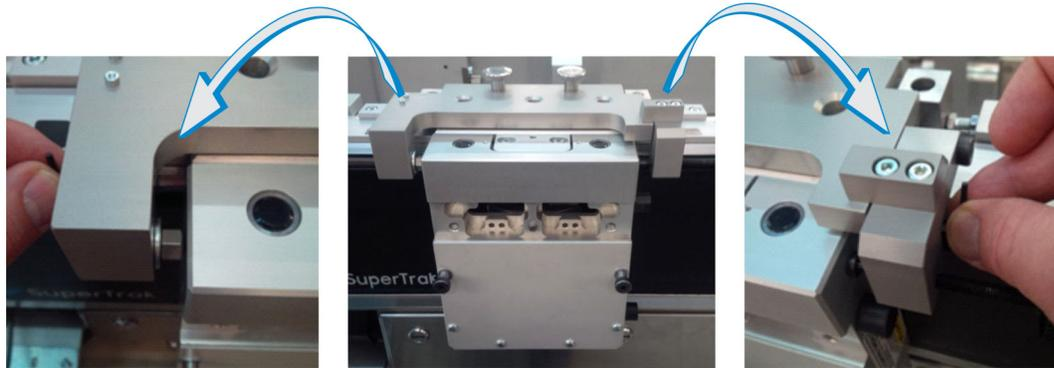
7. Turn the hex key(s) the required amount in the required direction to correctly adjust the encoder strip assembly. Aim for a shuttle position that is within a few microns; the value on the TrakMaster screen should be green.
