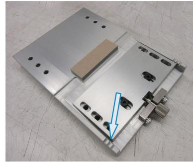
*NOTE: When assembling wedge adjusts, so that further adjustments can be made in both directions as needed, do not fully loosen or tighten the adjustment knob. The diagrams below demonstrate the correct spacing for the adjustment knob.*
