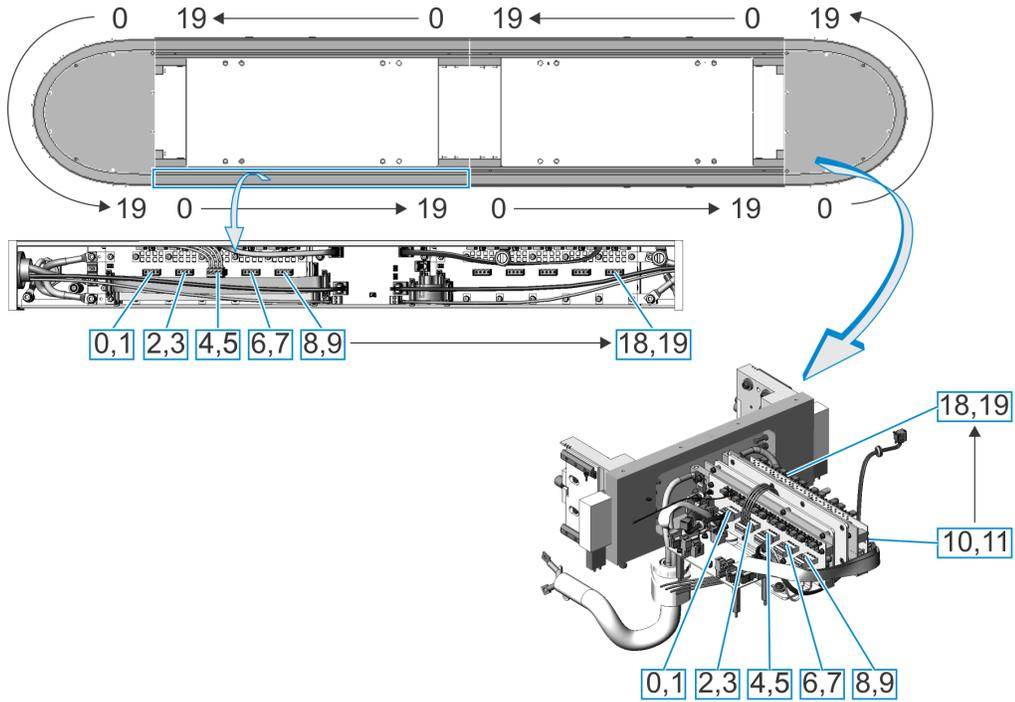
Each 180 deg. section (800 mm) has thirty (30) coils. The functionality is the same as described above except that the 180 deg. section (800 mm) has three (3) coil driver boards. As shown, the coils are numbered 0 to 19, and then 0 to 9 from left to right.
