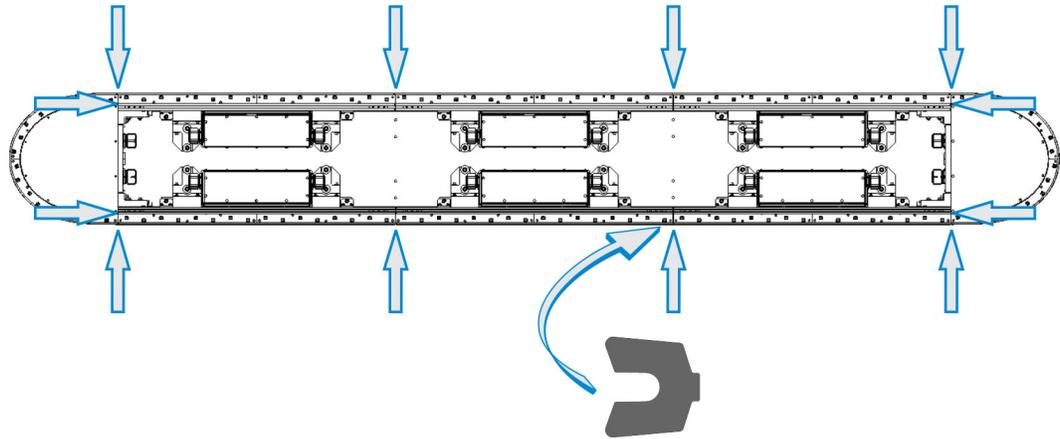
8. Install the wedge adjust for the 180 deg. sections. Place the precision level on the t-slot behind the encoder assembly of the straight section when leveling.
