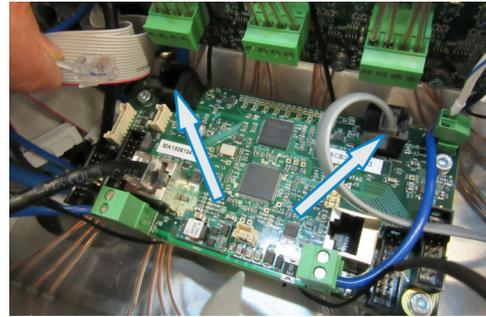
7. As required, unplug one (1) or two (2) motor network connection cables.
