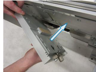
4. Loosely install eight (8) washers and eight (8) screws to install the wedge to the t-bars.
