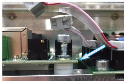
5. Secure the Gateway board in position with four (4) screws. To prevent distortion of the Gateway board, tighten one (1) screw at a time, working around the board in a clockwise direction.
