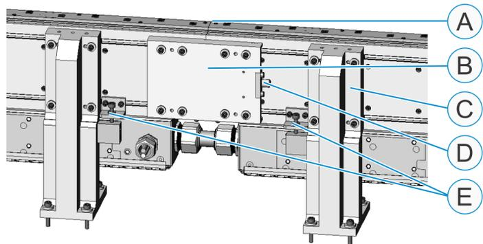
1. Choose a track section on which to base alignment for other sections as a starting point, then tighten all eight wedge screws on that section.
