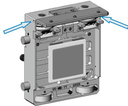
3. Remove the two (2) screws, two (2) lock washers, and two (2) flat washers that secure the shuttle encoder strip assembly in position.
