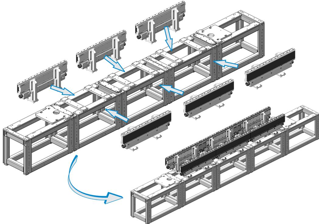
5. Push each straight section toward the center of the frame, so it is tight against the dowel pins in the frame.
