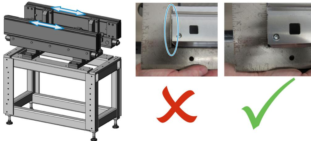
6. Tighten the four (4) screws at the base of each straight section stand.
