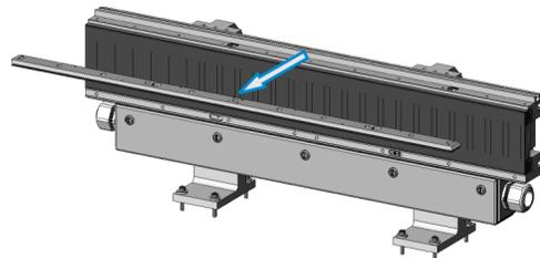
7. Clean the top of the straight section with a soft cloth to remove any debris.
