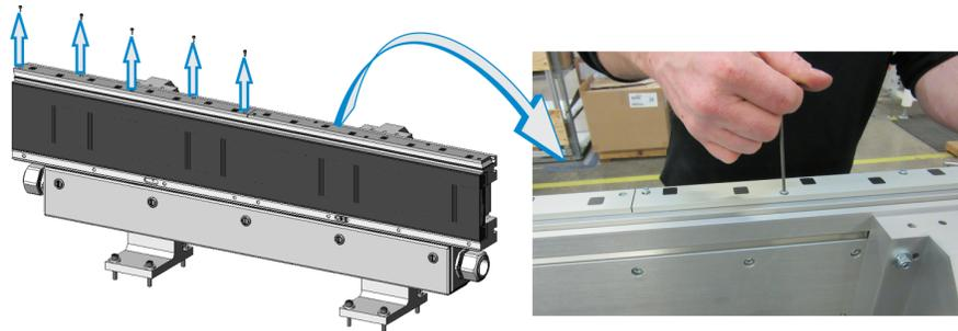
4. Remove the five (5) encoder assembly screws.
