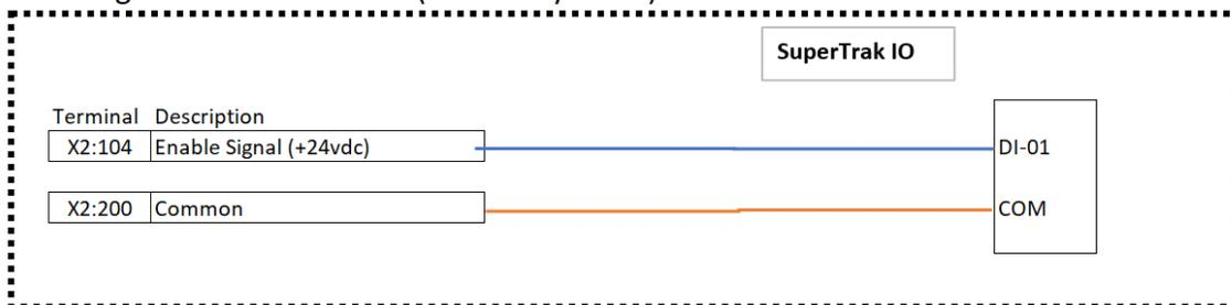
When not using the hardwired immediate stop signal, ensure there is a jumper between X2:103 and X2:104, as illustrated in the graphic below.
