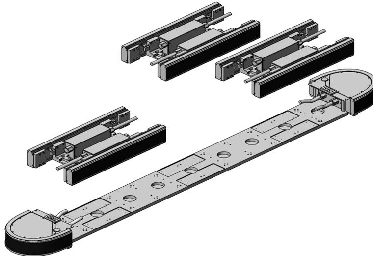
5. Loosely install four (4) screws into each straight section stand base. It is very important that the screws are centered in the screw holes as much as possible. This allows for adjustment when sections are connected together later.
