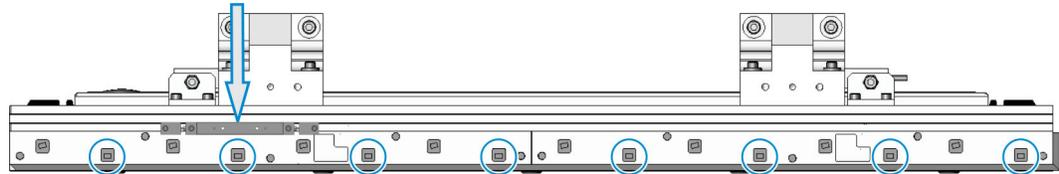
2. Install shims between the encoder assembly and the stationary mount, to bias the stationary mount to the back of the t-slot.
