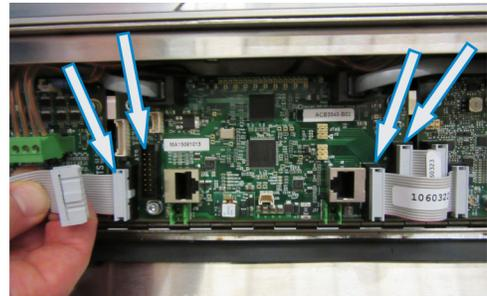
7. Disconnect the two (2) encoder cables (right and left).
