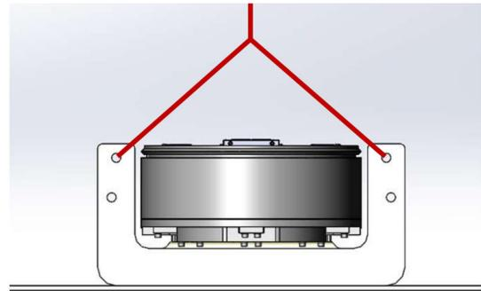
2. If required, reposition lifting brackets so that the mounting holes needed to attach the conveyor to the frame are accessible. Move shackle to the upper of the lifting holes on one side only.
