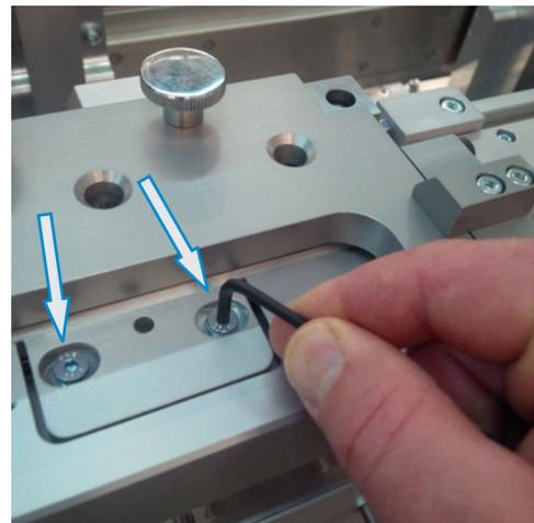
6. On each side of the encoder strip assembly, insert a hex key into the hole and engage the recessed set screw.
