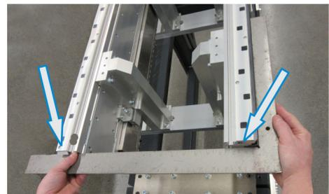
5. If the two (2) straight sections were not aligned in step 4, gently tap the straight section left or right (as required) until they are aligned.
