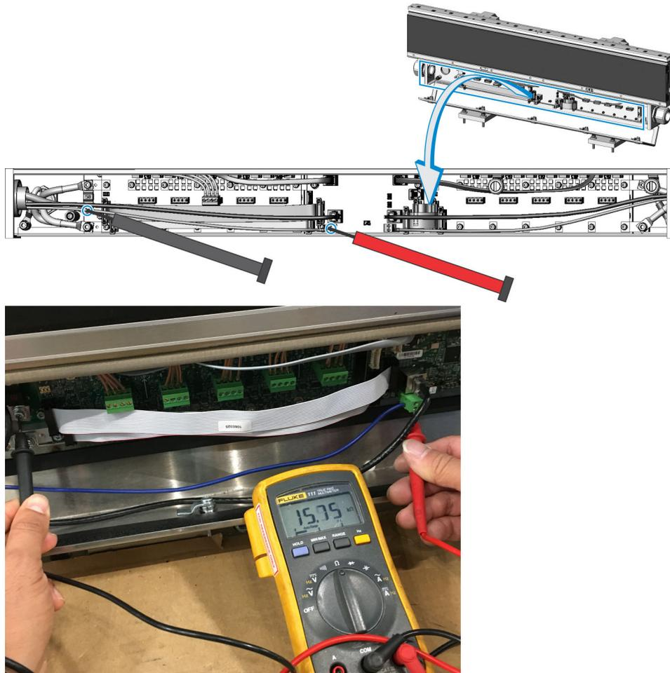
2. Look at the value displayed on the multimeter screen and determine if the resistance is acceptable:
