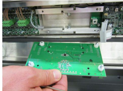
10. If the Gateway board is being returned for repair, remove the hardware (screws, washers, and spacers), and make sure the Gateway board is packaged in an ESD safe bag.
