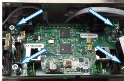
4. On each of the four (4) corners of the Gateway board, verify that the Gateway board sits flat on the white plastic spacers.
