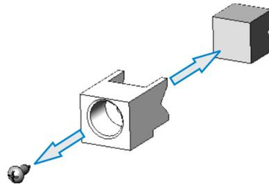
6. Position a new lubrication felt into the lubrication holder.
