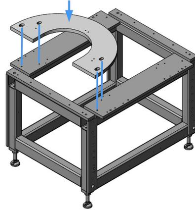
b. Install four (4) screws to secure the 180 deg. plate in position.
