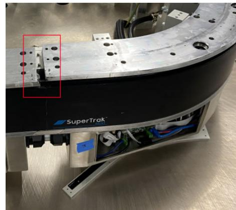
7. Slide the upper v-rail out in the forward direction clear of the motor.
