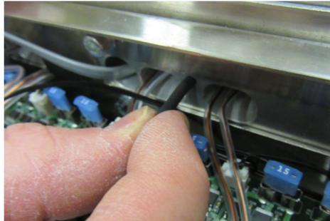
7. Slide the end of the new thermistor wire into the thermistor hole until you feel resistance.
