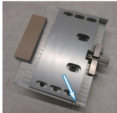
2. Place the magnetic shunt into the opening between the two (2) SuperTrak conveyance platform sections.
