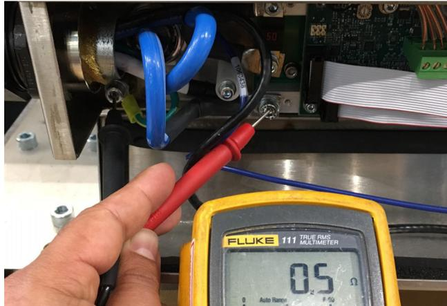
2. Look at the value displayed on the multimeter screen and determine if the resistance is acceptable:
