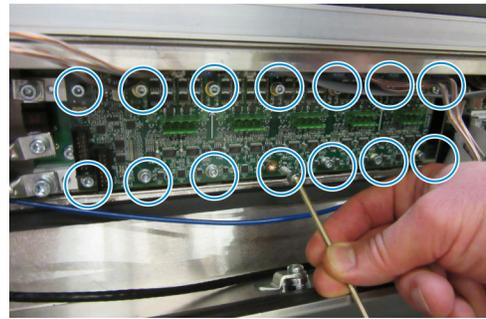
7. Pull the coil driver board straight down and out, and then disconnect the five (5) thermistor connections.
