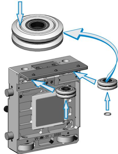
3. Align the spacer and v-wheel holes with the holes in the shuttle body.
