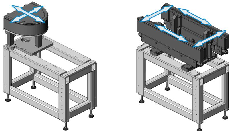
If the section is not level, adjust the required leveling screw.
