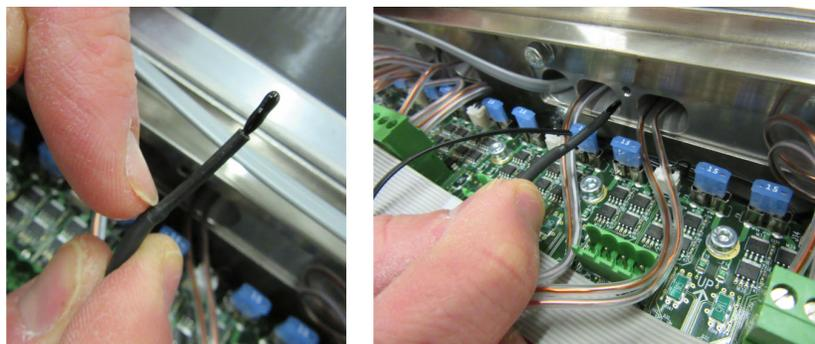
8. Plug the new thermistor connector into the electrical board.
