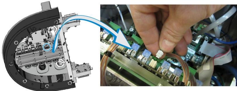
4. Unplug the thermistor connector from the coil driver board.
