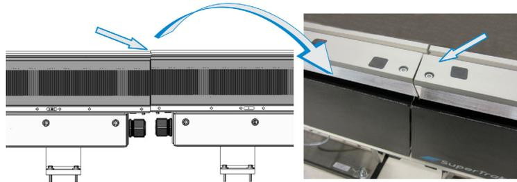
The image below illustrates a possible validation process, where two (2) indicators are mounted to a shuttle to measure the offset between the two (2) upper v-rails.
