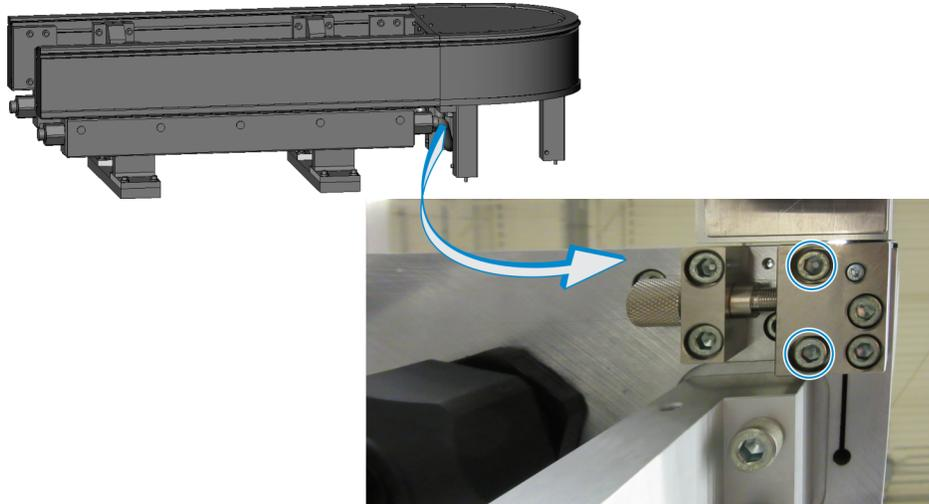
2. Turn the adjustment knob as required, until the flat wear strip on the curved section aligns with the flat wear strip on the straight section.
