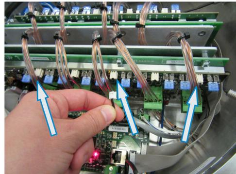
8. Lean the coil driver board forward and lift straight up.
