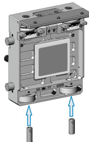
6. Fully remove the set screws, to verify that the flat of the shaft is aligned with the set screw.
