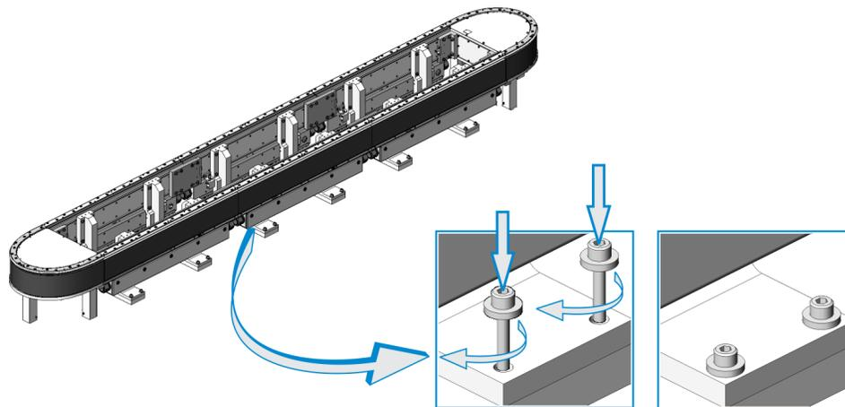
25. For 180 deg. (500 mm) sections only, reinstall the sections' top covers, and then reinstall the stand covers.
