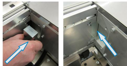
Slide the magnetic shunt into the opening width-wise, and then push it sideways into location. Do not place any objects in the opening before the magnetic shunt is inserted. The magnetic shunt requires iron-to-iron contact with the motor core of both the straight section and the curved section.
