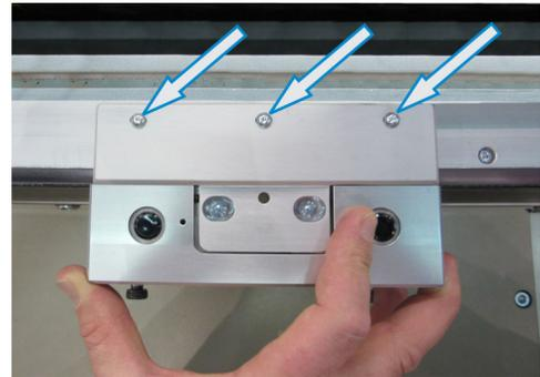
4. Install an M2.5 x10 mm screw into each side of the shuttle encoder strip assembly.
