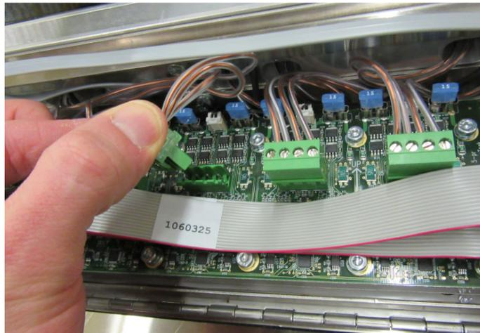
5. Unplug the thermistor connector from the coil driver board.
