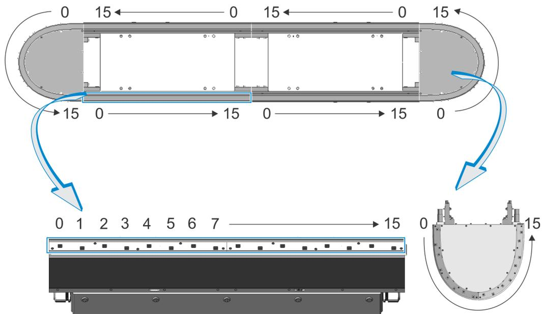
Each 180 deg. section (800 mm) has four (4) encoder assemblies: a left encoder assembly, two (2) center encoder assemblies, and a right encoder assembly. The functionality is the same as described above except that the encoders are numbered 0 to 7 from left to right, as pictured at right.
