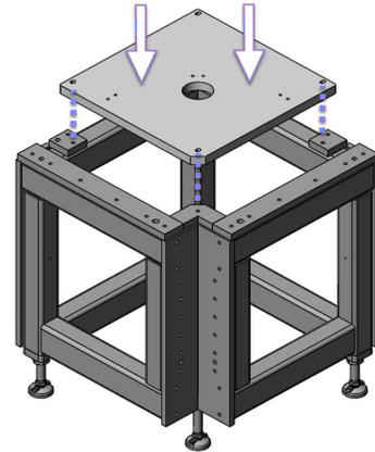
*NOTE: When the overall conveyor arrangement is longer than it is wide, orient the mounting plates so that the slots align with the long axis of the conveyor.*
