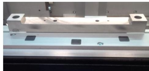
4. Snug the two (2) stationary mount screws. Make sure the t-nuts turn and lock into the t-slots.
