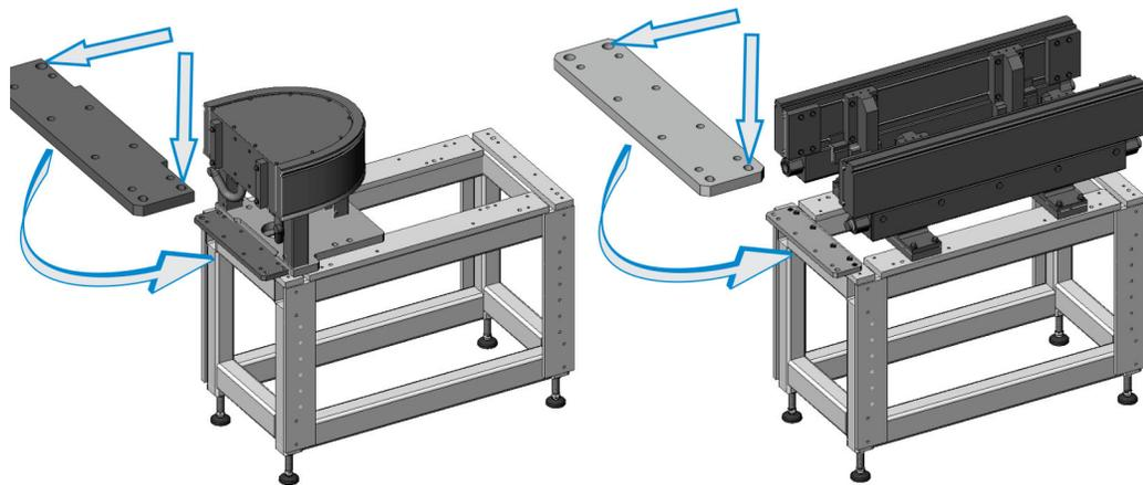
*NOTE: If you are using compact frames to support 180 deg sections, use the supplied stepped dowels to attach the connector kit to the joint between the compact frame and the one-meter section frame, as pictured.*
