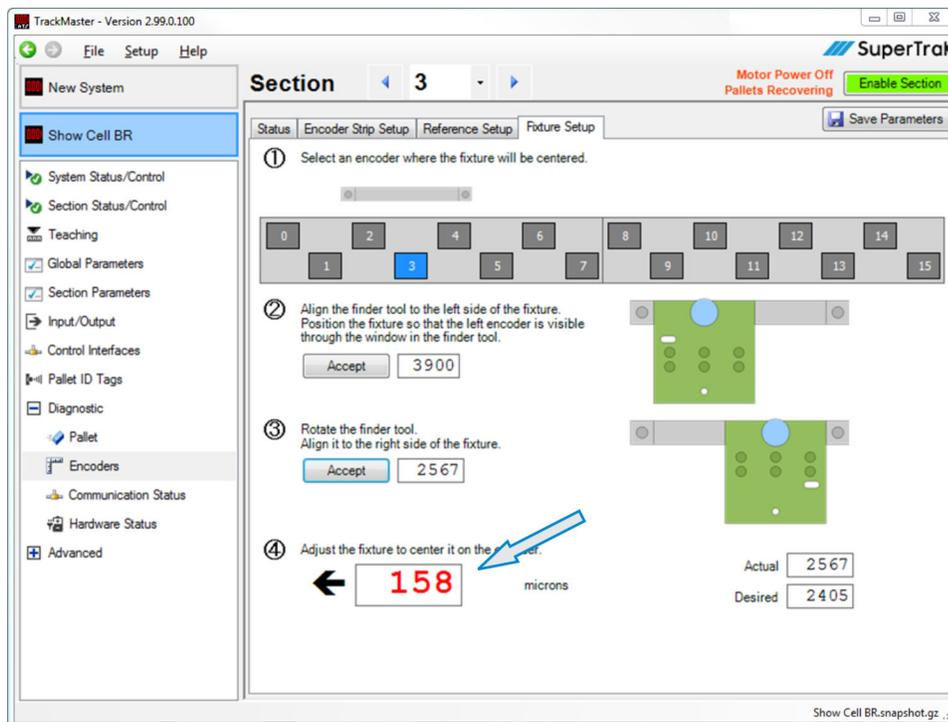
11. As required, adjust the position of the shuttle setup station locate:
