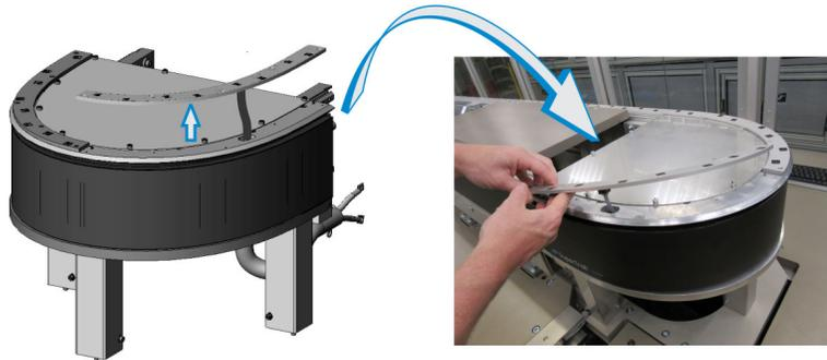
6. Disconnect the RJ11 plug from the encoder assembly connection.
