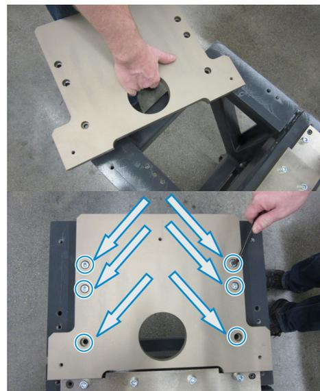
3. Loosely install one (1) lock washer, and one (1) screw in each of the three (3) stand bases.
