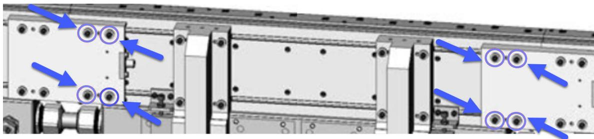
2. Now tighten the four wedge screws on the next section over.
