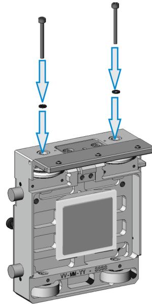
7. Install a plastic cap over each of the two (2) screws.
