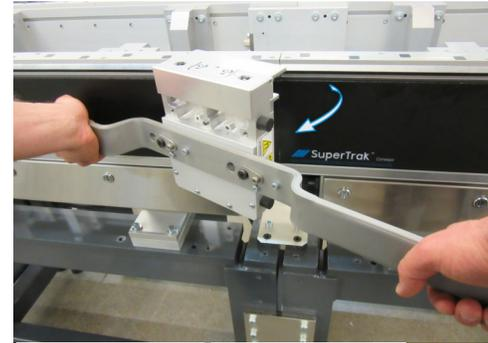
4. Slide a keeper plate over the shuttle magnet assembly with the polycarbonate side of the keeper plate against the shuttle magnet.
