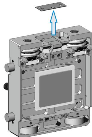
8. Measure the current combined shim thickness.
