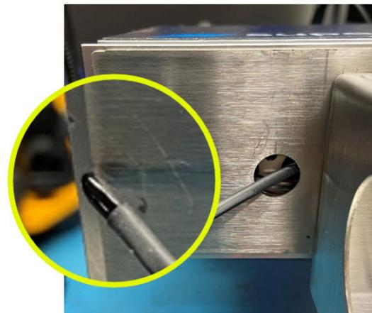
6. Thread the wire with the new thermistor back through the hole in the cabinet.
