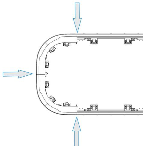
18. Adjust the vertical, horizontal, and side-to-side positions until the upper v-rails align with the straight sections, and the curved section is centered between the straight sections.
