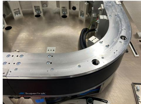
4. Remove fifteen (15) screws from the upper v-rail, and remove the screws from the adjacent sections as well.
