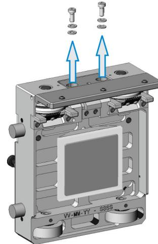
4. Lift and remove the shuttle encoder strip assembly.
