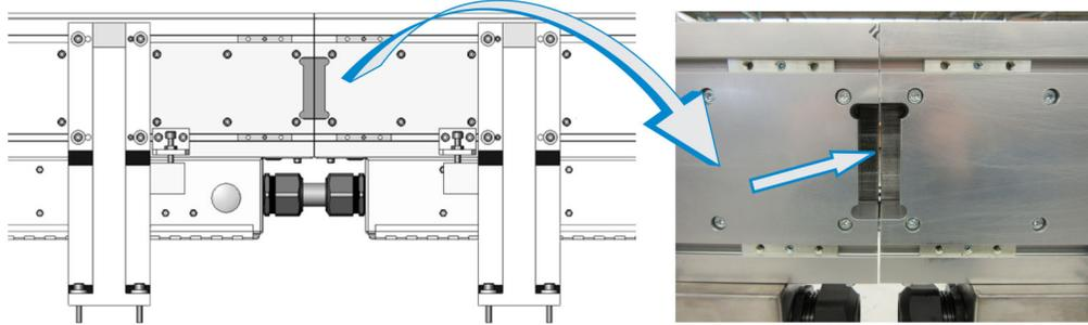
The image below provides a top view of two straight sections that are not aligned.
