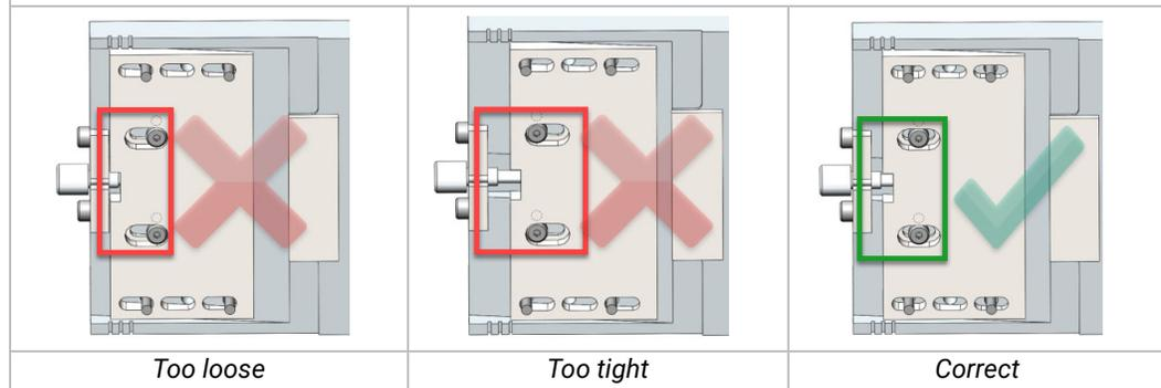
2. Place the magnetic shunt into the opening between the two (2) straight sections.
