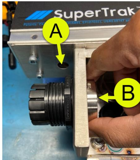
4. Once the electrical interconnect is removed, look for the motor thermistor and wire through the hole in the cabinet. Use needle-nose pliers to gently pull the wire through the hole.
