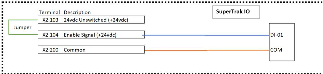
In both immediate stop signal diagrams above, X2:104 corresponds to SuperTrak Digital Input 0, which is configured in TrakMaster as "Allow Section Enable" by default. See TrakMaster Help, Digital I/O Configuration for more information.
