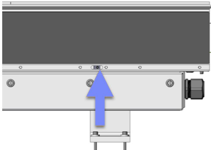
17. Install the wear strips to the straight sections.
