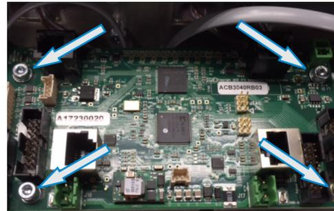
6. Torque each of the four (4) screws to 18 lbf-in (2 Nm).
