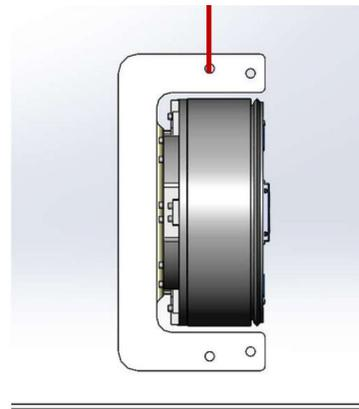
6. Once this change in orientation is complete, mount to frame and then remove lifting bracket (or store in the vertical orientation).
