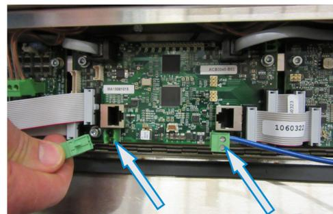
5. As required, unplug one (1) or two (2) motor network connection cables.
