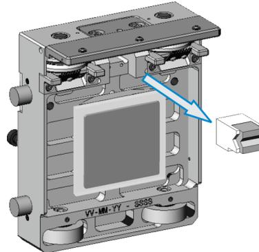
5. Remove the screw from the back of the lubrication holder, and then remove the lubrication felt from the lubrication holder.
