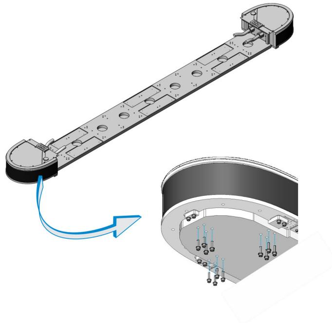
4. Mount the straight sections with their electrical boxes facing inwards, starting with the sections closest to the 180 deg. sections.
