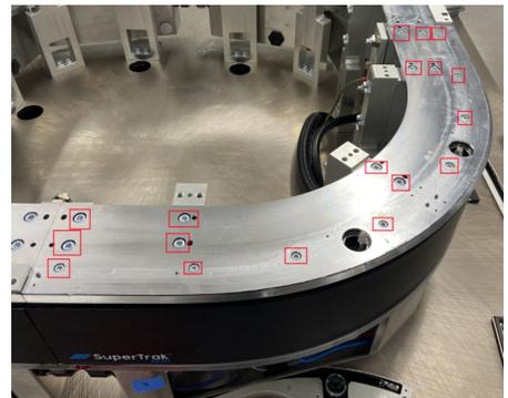
5. Note the position of the 0.25 mm (0.01 in.) shim, and then place the shim in a safe location.
