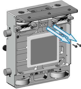
3. Remove the lubrication locking block.
