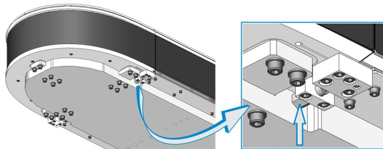
15. Tighten the four (4) screws in each straight section stand base.
