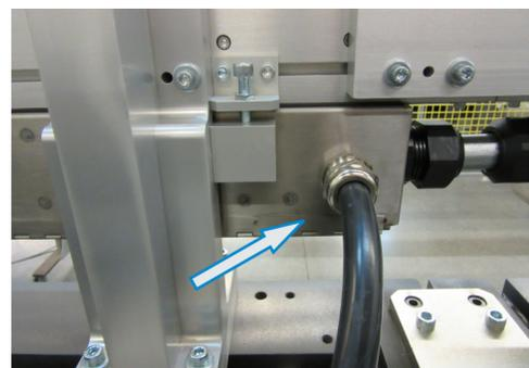
8. Connect the power supply cables to the left coil driver board:
