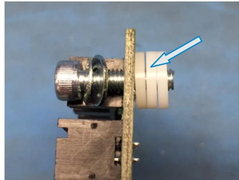
3. Align the screws in the Gateway board with the threaded holes inside the straight section.
