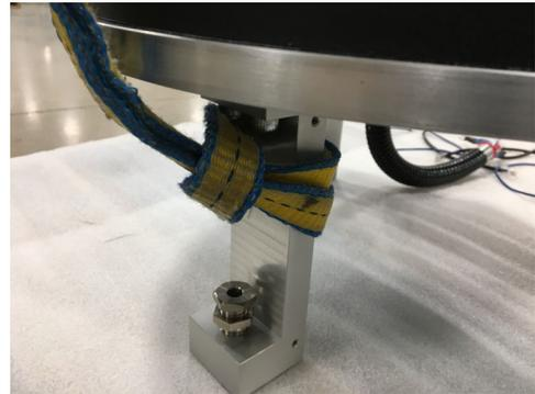
2. Use an appropriate lifting device, such as a forklift, to lift the 180 deg. section up by the ends of the lifting straps.
