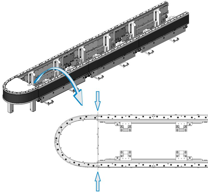
For 90 degree sections, use shims to verify that a 0.5 mm (0.02 in.) gap exists between the 90 deg. section and each of the two (2) abutting sections.
