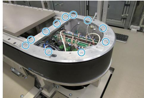
7. Lift the top plate straight up to remove it.
