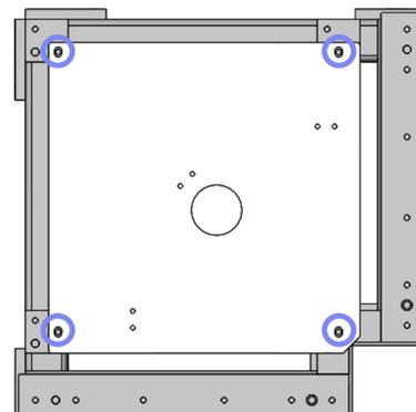
2. Lift and position a 90 deg. section on the 90 deg. plate.
