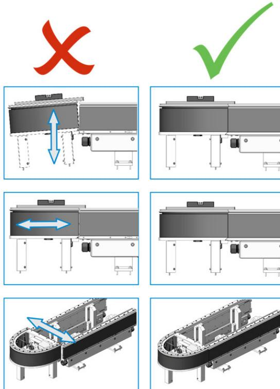
For 180 deg. (500 mm) sections: Remove the top cover from the 180 deg. section, remove the covers from the 180 deg. section stands, and then level the 180 deg. section.
