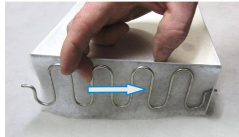
2. Remove the filter retention clip.
