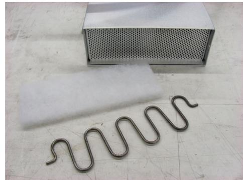
5. Position a new filter into the base of the power supply.
