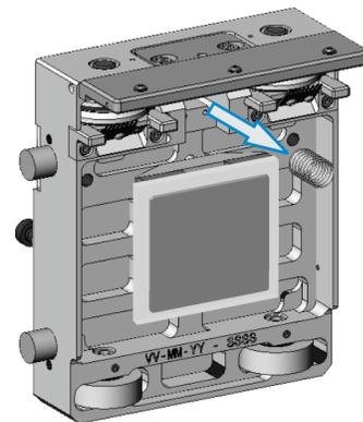
3. Position a new spring into the shuttle.
