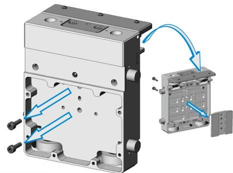
6. As required, secure the 2-magnet assembly in position with two (2) screws, or the 3-magnet assembly with four (4) screws.
